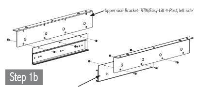
Lower Side Bracket RTW/Easy-Lift 4-Post, PedSys, left side
